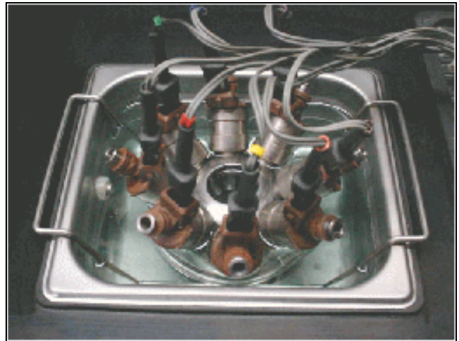
Ultrasonic cleaner. Note injectors are wired to be active during cleaning.
