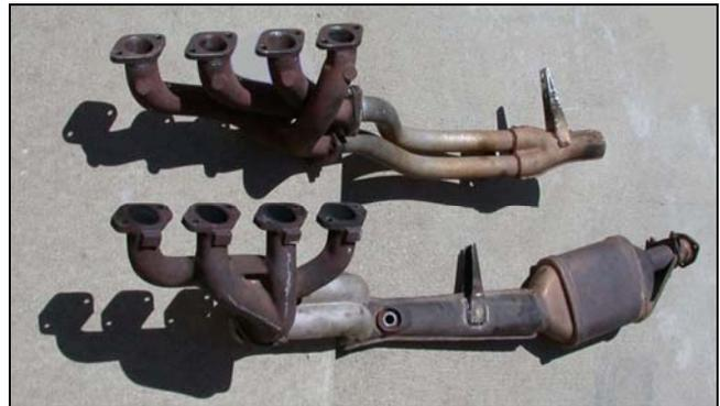
Martellina's old system (bottom) and new system without its converter. Photo by Elio Comello.
