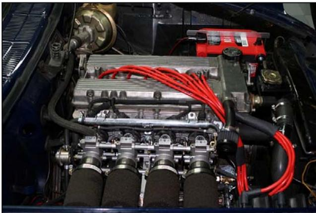
The next step was wiring up the ECU and all the extra bits. The ECU controls the injectors, the ignition, the electric fan, a shift light, the coils and the fuel pump. It can also control idle air, but I did not use this feature. Normally on a FI motor the ECU opens a valve to let air in if the idle speed drops below a set rpm. I used spark advance control to do the same thing. If you have ever adjusted a distributor
