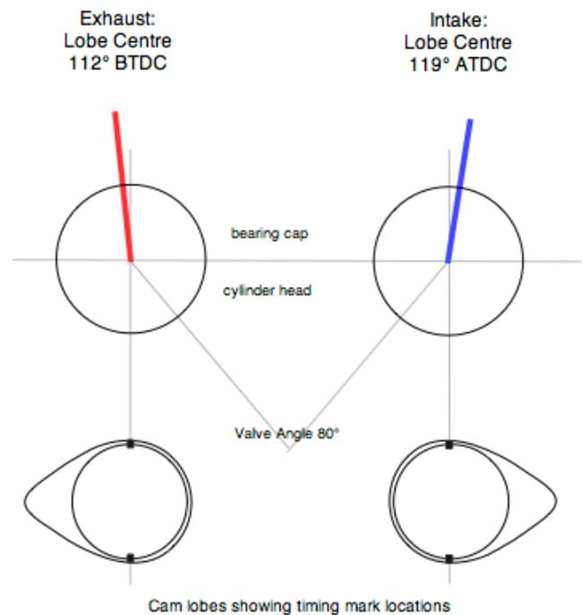
N.B. Direction of rotation is counter clockwise as seen from the back.
