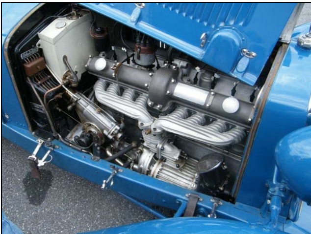
A beautifully prepared engine compartment. It too has a gasoline surge tank. Photo by George Beston.
