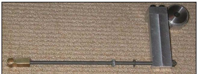
*The brass fitting at the top fits over a bolt threaded into the face of the front air plenum adaptor.*
