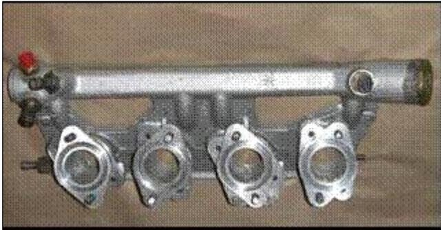
The aluminum mounts have the secondary benefit of eliminating the support strut between the engine mount and intake plenum. The benefits that the rubber mounts provide, i.e. isolation from heat and vibration, are not required for fuel injection systems, so nothing has been lost.
