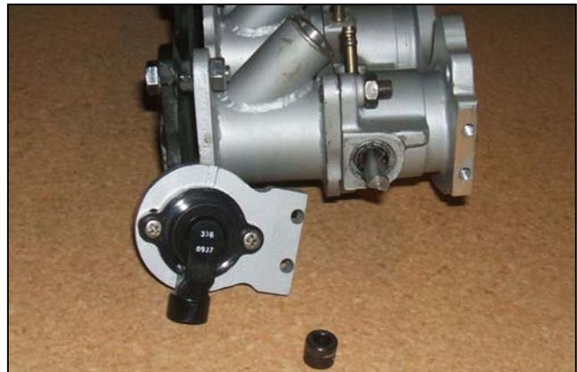
Finally, air distribution blocks were taken from two Spica systems for idle air and MAP (Manifold Absolute Pressure) signal purposes. A needle valve was included on the MAP side to damp out signal spikes. An adjustable throttle stop was required to establish a base idle, and a throttle return spring
