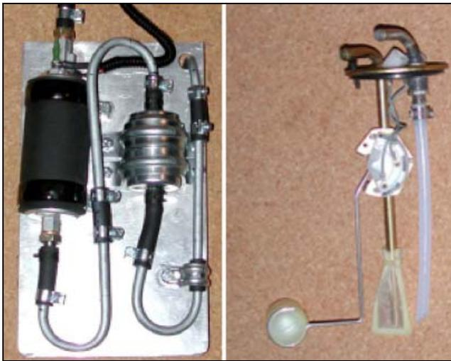
*Above left: Fuel pump, primary filter and mounting plate.*
