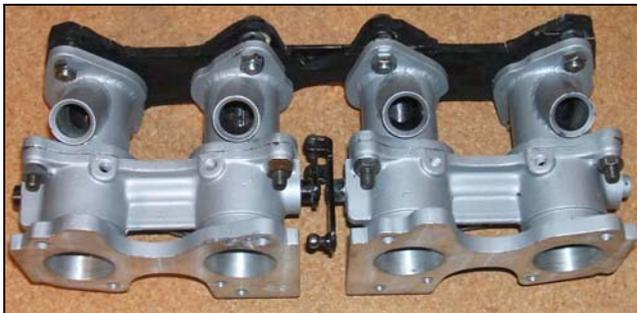
Starting with flanges scalped from used rubber carburetor mounts, then using custom made parts to build up the injector bosses and finally making adapter plates to bolt to the original die-cast air
