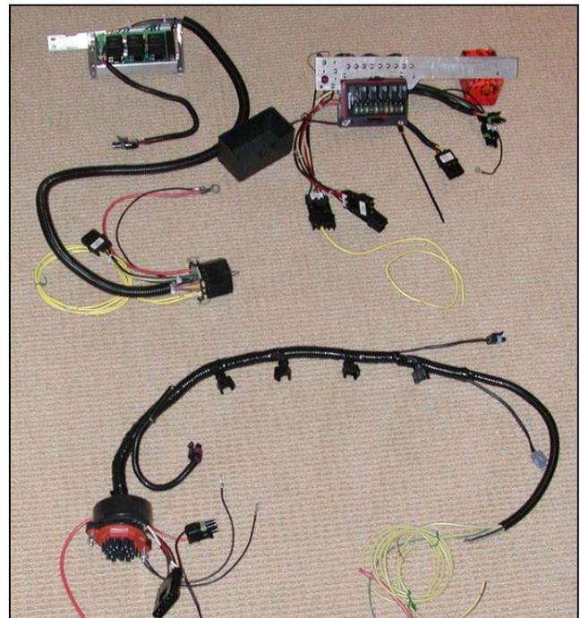
*Clockwise from top left: Relay board and interior harness; auxiliary fuse/relay box; engine compartment harness.*
