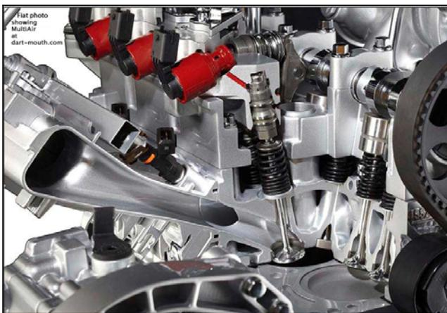
MultiAir Intake Cutaway. Fiat image from Dart-Mouth.com
