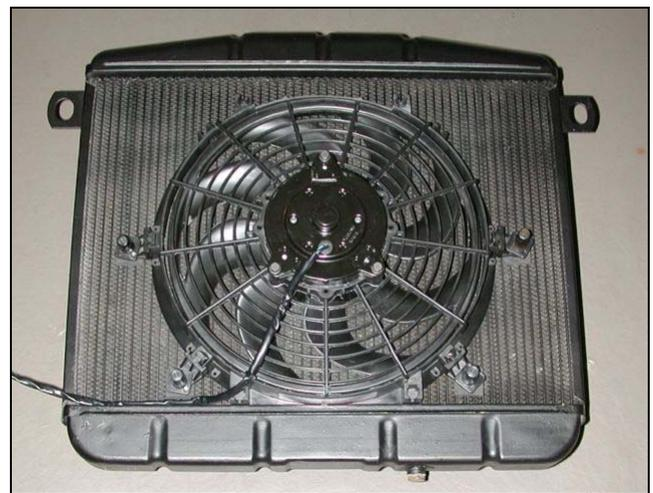
*Electric fan on cleaned and re-painted radiator.
