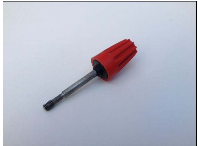
Modified fuse box cover bolt. Photo by Russ Baer.
