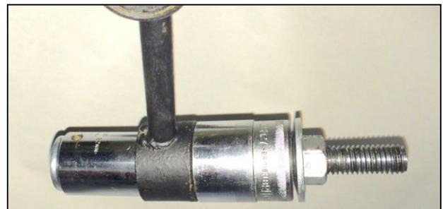
*This picture shows the tools assembled and ready to start tightening the nut to pull the bushing out of the dog-bone. Photo by George Beston.*
