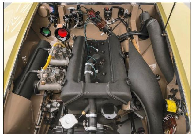
Accentuating its sporty pretensions, the car was fitted with a competition-style Tipo 1308 engine with large-diameter valves, a ram-type induction system of the type found on period Ferrari four-cylinder racing cars, and twin high-volume Weber 50 DCO3 carburetors, as well as a five-speed transmission.
