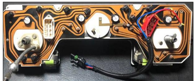
The following image shows the finished results. The only surprise after all the bench testing was that the LED dimmer has no effect unless more than 12.5 volts are available from the electrical system.
