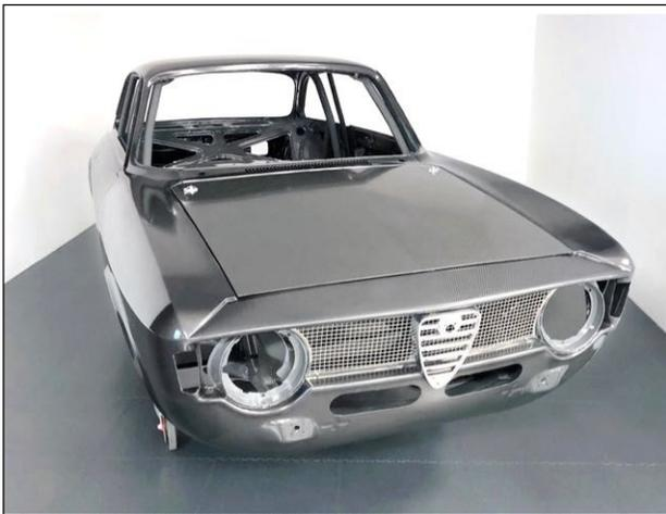
This body reportedly saves 70 kg over a steel-bodied version and 38 kg over a GTV body fitted with carbon fibre hood, trunk lid and doors.
