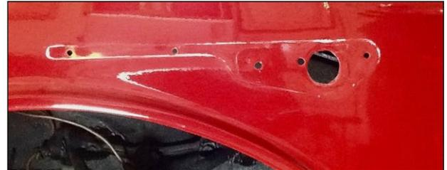
The two elements went together well and the wiring was straight forward. The socket and wiring are exposed in the wheel well so it's easy to understand why the original socket was in poor shape.
