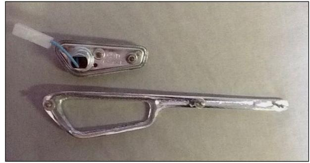
with the screws held in place by soldered on 'cages', allowing a bit of wiggle room. The new trim was a casting with the screw bosses rigidly cast in place.
