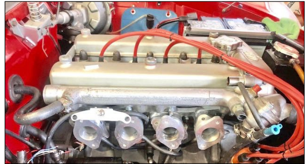
Mounts in place and vacuum system assembled. A needle valve to dampen vacuum fluctuations is located above carb mounts 3 and 4. Photo by George Beston.
