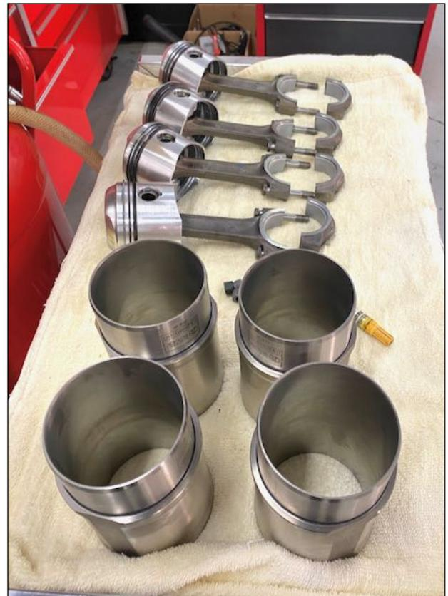
*Here, the pistons and connecting rods are assembled waiting for the liners to go in.*
