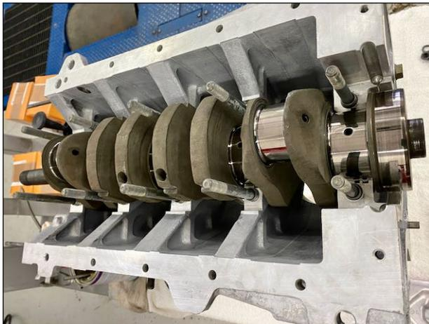
*The crank shaft in place waiting for main and rod bearings.*
