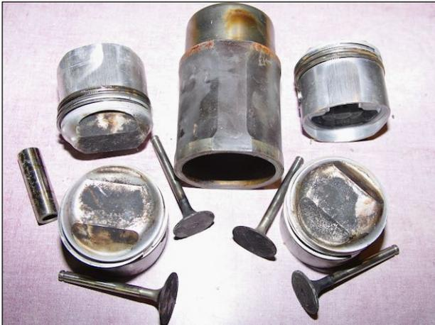
*Some old parts; pistons, valves, a liner and a wrist pin. Note the scoring on at least two of the pistons.*
